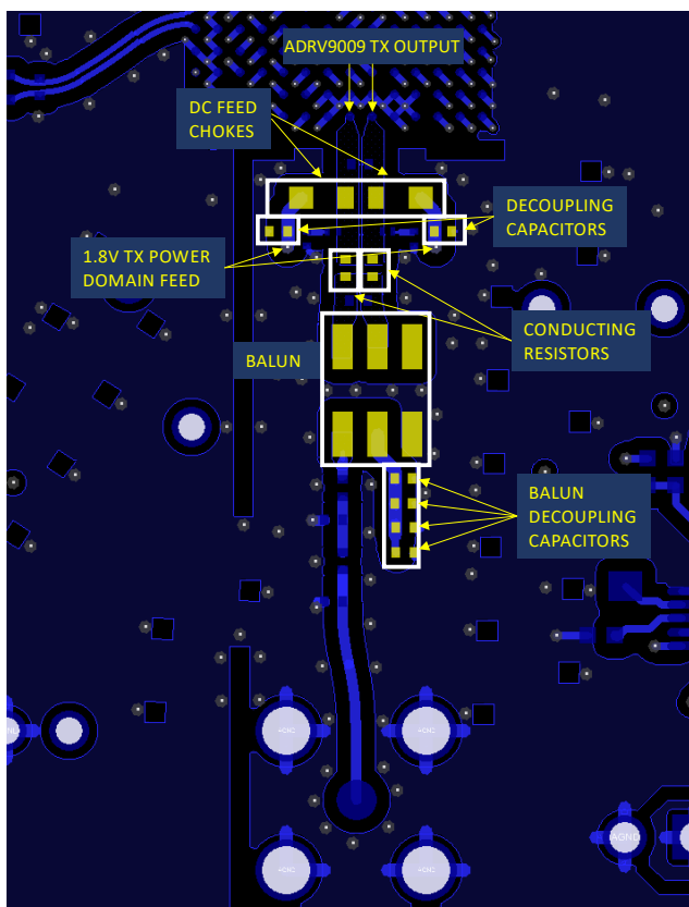
Figure 443. Transmitter DC Chokes and Balun Feed Supply
